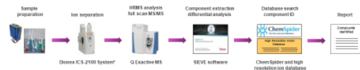
Figure 1. Ion exchange chromatography and high resolution mass spectrometry workflow for lithium-ion battery anode impurity analysis
