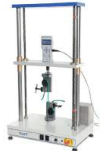
Motorized machine with force and displacement measurement
