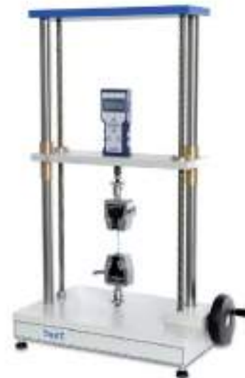
Manual bi-column machine with force measurement
