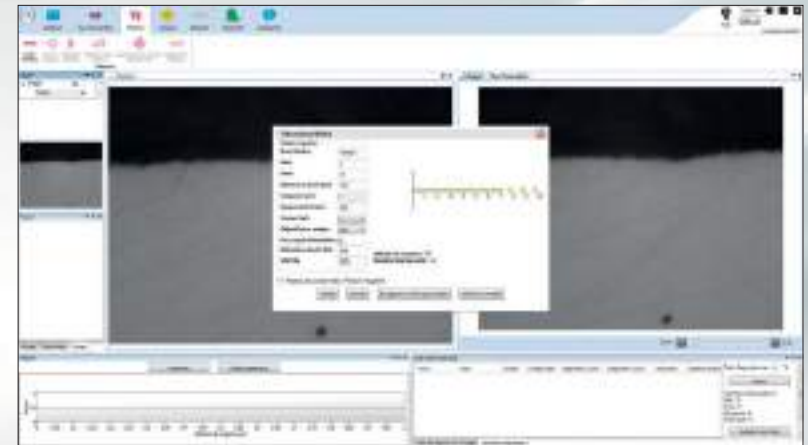
PRESI Touch Manual Pattern creation. A graphic and dynamic assistant allows pattern visualisation during its programming.
