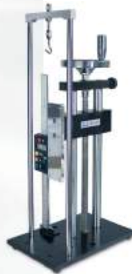
Manual machine with force and displacement measurement
