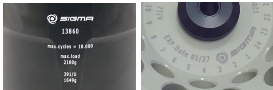
Fig. 5: Different service life – engraving on the bucket/rotor
