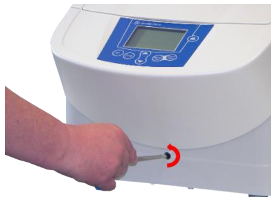
Fig. 11: Manual release of the lid lock
