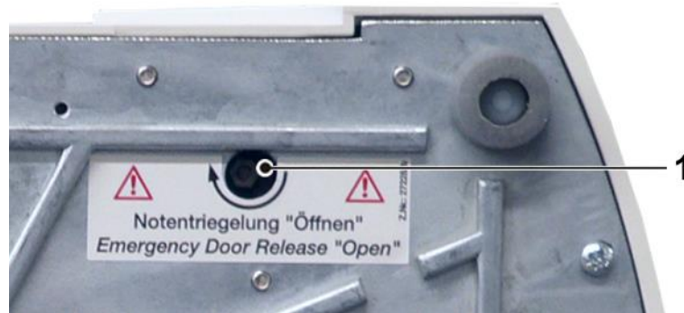
Fig. :14 Opening for the emergency lid release at the bottom of the centrifuge
