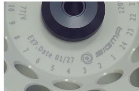
Fig. 4: Different service life – engraving on the bucket/rotor
